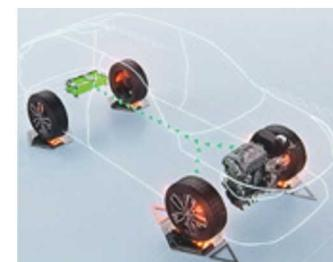
**Regenerative braking** uses the energy generated by the electric motor when braking to recharge the main drive battery
