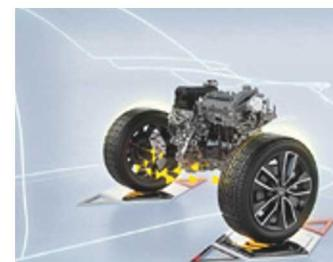
**Engine drive** uses the petrol engine to maintain higher cruising speeds – during motorway or open road driving, for example
