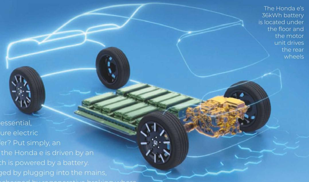
It's a common, but essential, question: how do pure electric and hybrid cars differ? Put simply, an electric car such as the Honda e is driven by an electric motor, which is powered by a battery. The battery is charged by plugging into the mains, but it can also be recharged by regenerative braking where the car's motion is used to generate electricity as it slows.
